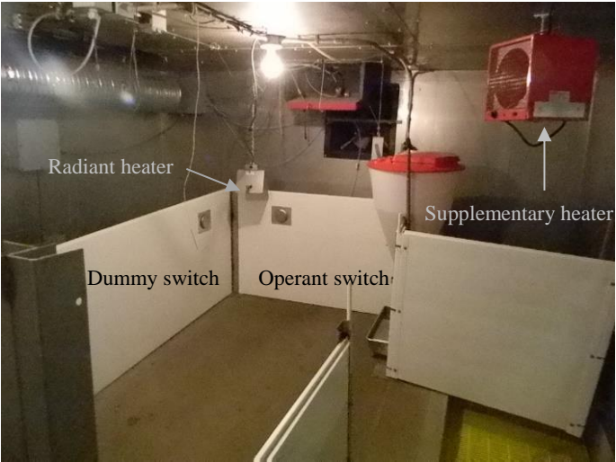
Figure 2. Operant and dummy switches installed on the penning and radiant heater fixed from the ceiling in each of the identical chambers.
