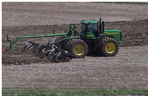
Figure 2. PCE manure application system.
