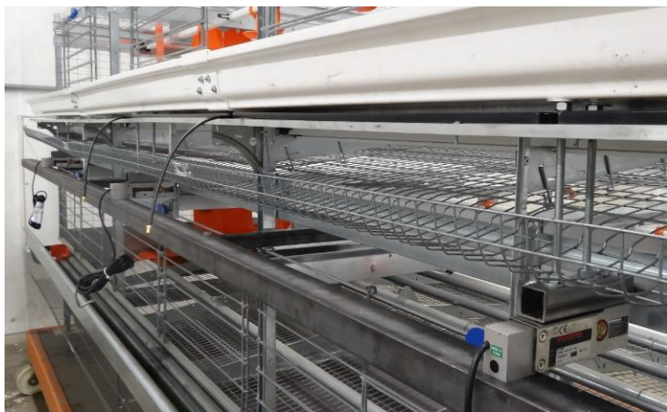
Figure 7. Feed intake measurement system. A plastic feed trough is connected to three load-cells placed under the egg collection rack and supporting the feeder through the vertical bolts.
