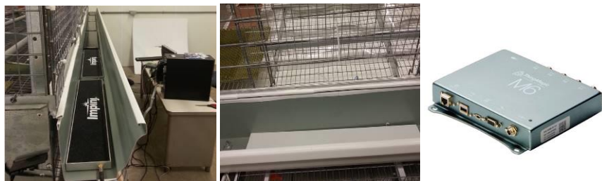
Figure 8. The RFID antennas placed inside the feed trough (left), covered with plastic plate (middle), and the reader (right) used to monitor feeding behaviors of individual birds.
